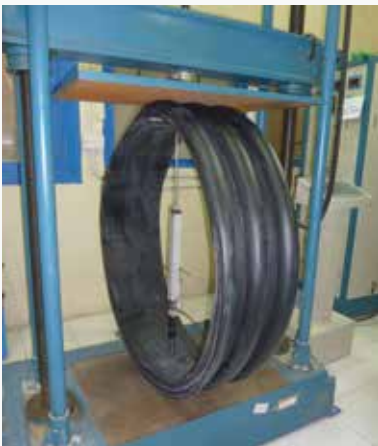
Ring stiffness testing as per ISO 9969
